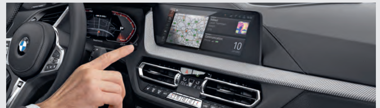
With BMW Gesture Control , selected functions can be operated by means of defined hand movements. Simple gestures such as 'swiping' or 'pointing' are identified in the recognition area above the centre console and trigger functions such as accepting or rejecting an incoming telephone call, proceeding or cancelling navigation as well as starting and ending voice recordings.
